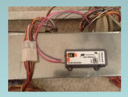
New 20K sensors with new or old wiring
