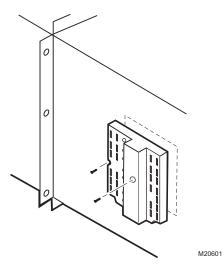
Fig. 30. Mounting the module on sheet metal.
