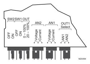
Fig. 37. C7232 default jumper settings for models with date code prior to 0309.
