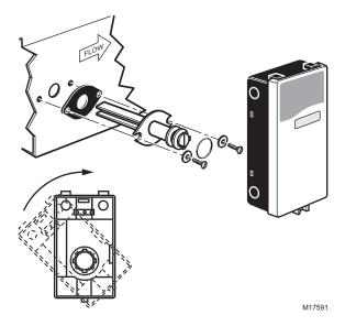
Fig. 13. Duct mounting (C7232B).
