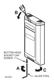
Fig. 11. C7232A cover removal.
