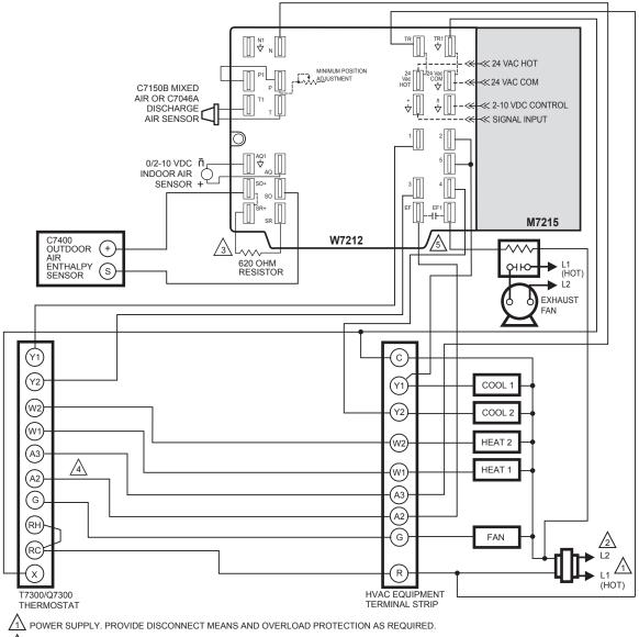
$ot\! \Delta$  ensure that transformer is sized to handle the extra load of the economizer and actuator.
