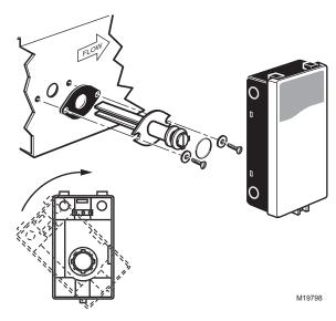
Fig. 22. Duct mounting (C7632B).
