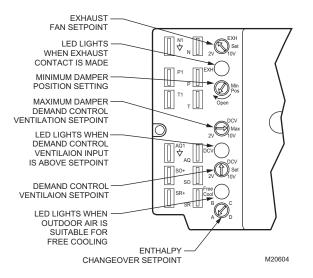
Fig. 33. Potentiometer and LED locations.
