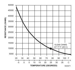
Fig. 8. C7150B1046 Sensor resistance temperature.
