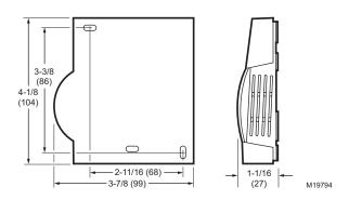
Fig. 18. C7632A dimensions in in. (mm).
