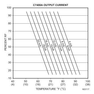
Fig. 17. C7400A Sensor output current vs. rh.
