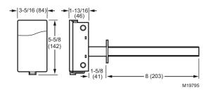
Fig. 19. C7632B dimensions in in. (mm).
