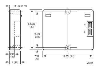
Fig. 16. Approximate dimensions of C7400A Solid State Enthalpy Sensor in in. (mm).
