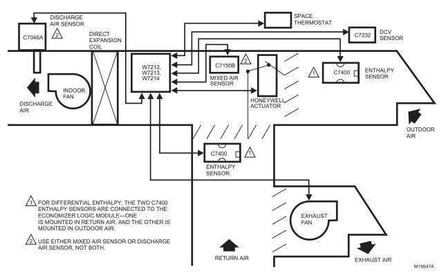
Fig. 31. Representative locations of connected economizer system devices.
