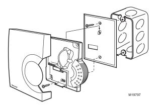
Fig. 21. Junction box mounting (C7632A).
