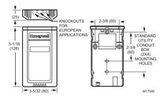
Fig. 9. C7232A dimensions in in. (mm).
