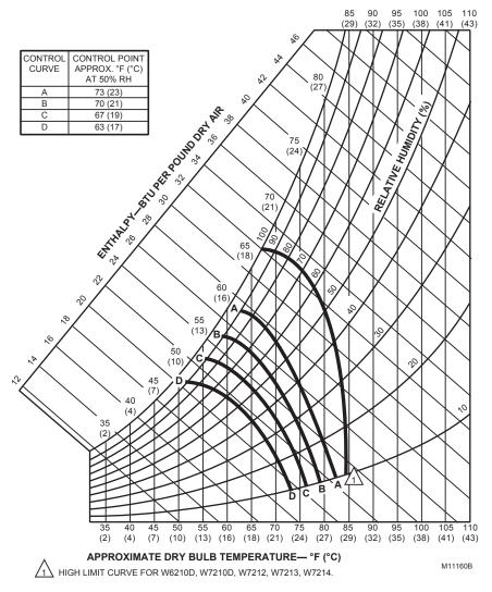
Fig. 34. Partial psychrometric chart with single C7400 Solid State Enthalpy Sensor and W7212 Solid State Economizer Logic Module performance Curves.
