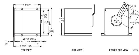
Fig. 26. M7215 Damper Motor dimensions in in. (mm).
