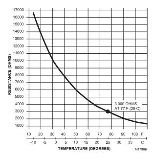
Fig. 4. C7046C Sensor resistance vs. temperature.
