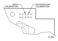
Fig. 24. C7632 calibration pads.
