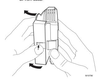
Fig. 20. C7632A cover removal.
