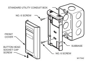
Fig. 12. Junction box mounting (C7232A).
