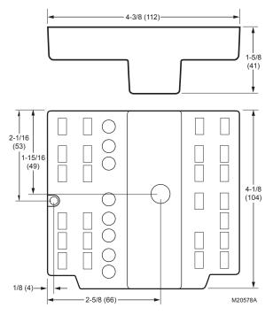
Fig. 28. Logic module dimensions in in. (mm).
