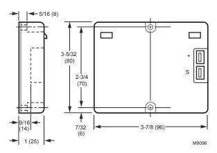
Fig. 25. C7650A Thermistor Temperature Sensor Dimensions in in. (mm).
