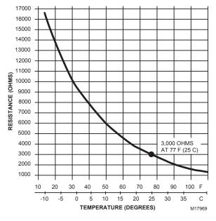
Fig. 7. C7150B1004 Sensor resistance temperature.
