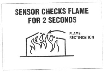
31. The molecules of burning gas flowing between the burner and sensor become ionized and capable of conducting electrical current. A pulsating direct current signals the safety logic when the flame is stable and strong. For the IGC to sense a stable, strong flame, .2 microamp is needed. The flame is sensed for 2 seconds to make the "go" or "no go" decision. This process is known as *flame rectification*.
