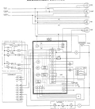
37. If the unit is equipped with an economizer, the fan logic signals the economizer through terminal IFO of J2 when the fan is running. The compressor contactor circuit is also routed through the economizer.
