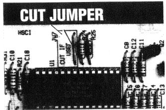
15. When a pressure switch or centrifugal switch is used, the jumper shown here must be cut. A cut jumper will signal the IGC that a pressure switch or centrifugal switch is to be used in place of a Hall Effect sensor.
