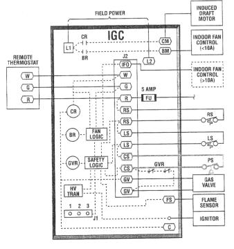
14. If the unit uses a pressure switch or centrifugal switch to prove the induced draft motor, the switch will be connected to terminal CS on J2 and will thus be in series with the other safety switches. On such units, the jumper across the CS terminals will be removed when the switch is installed.
