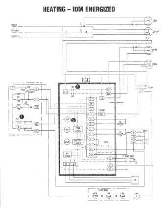
27. When there is a call for heating, the TH1 thermostat switch, at 1, closes to provide a path through terminal W to combustion relay CR, at 2. This energizes the induced draft motor (IDM) by closing the set of normally open CR contacts, at 3.
