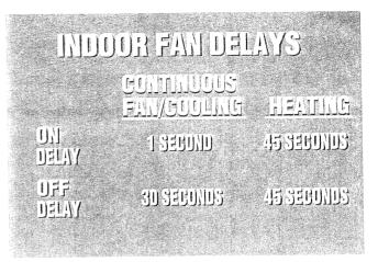
10. In the cooling mode, the fan logic activates the blower one second after the thermostat calls for cooling. This prevents the blower motor from starting at the same instant as the compressor motor(s) and outdoor fan motor(s). When the cooling thermostat opens, there is a 30-second delay before the blower shuts off, in order to take advantage of residual cooling capacity in the system. The continuous fan mode also has a 1-second on delay and a 30-second off delay.
