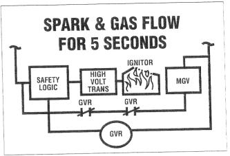
30. At the same time, the safety logic energizes the gas valve relay and its two N.O. contacts close to open the gas valve and light the burners. The contacts are wired in series so that a welded contact cannot result in an open gas valve. The gas and spark continue for 5 seconds.
