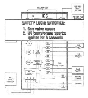
17. When the safety logic is receiving all the necessary inputs from the safety switches, fan logic, and induced draft motor sensor, it will open the gas valve and start the gas flow.
