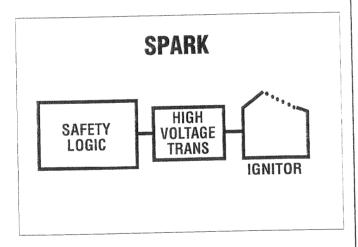
29. The safety logic signals the high voltage transformer to create a high voltage spark for 5 seconds. This is a 10,000-volt spark, so be careful when troubleshooting in this area.
