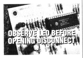
51. Remember to observe the display shown by the LED before opening the disconnect, so that any coded message is not canceled.
