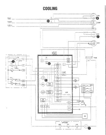
26. In the cooling mode, cooling thermostat TC1, at 1, closes on a call for cooling. This completes a path through Y1 to the compressor contactor C, at 2, assuming that all safety devices in the path are closed.
