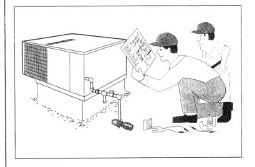
49. Keep in mind that the IGC diagnostic function only identifies system problems which might include the IGC board itself and that it does not resolve these problems. To resolve any problems, the service technician must apply standard trouble-shooting and service techniques, such as checking the supply voltage, "hopscotching" the power or control circuits, checking system components, and other commonly used service methods.
