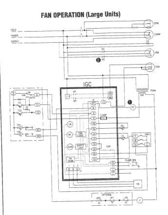
25. In larger units, the indoor fan contactor (IFC) contacts control the operation of the indoor fan motor, as shown here. The fan logic energizes indoor fan contactor IFC, at 1. Two sets of normally open IFC contacts, at 2, in the power circuit close to start the indoor fan motor. The on and off fan delays for the large units are the same as those for the small units.
