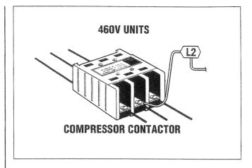
7. There are 208/230-volt and 460-volt versions of the IGC. The 208/230 version has an L2 connection on the board; the 460-volt version does not. A lead from the compressor contactor supplies the L2 voltage.
