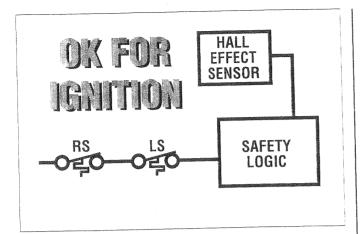
28. The IDM reduces the pressure in the flue collector box by drawing air and/or combustion by-products through the heat exchangers. When the IDM is running, the Hall Effect sensor (in this case) signals the safety logic. If the limit and rollout switches are closed, the safety logic will initiate the ignition sequence.
