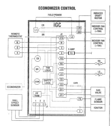
11. If the unit is equipped with an economizer, the IGC fan logic sends a signal through J2 terminal IFO to tell the economizer when the blower is on.
