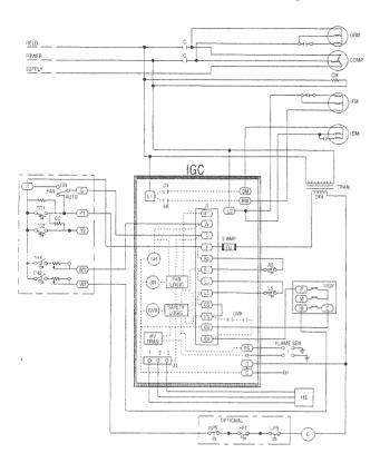
23. For our discussion, we have selected a typical heating and cooling unit with 208/230-volt three-phase power, a 24-volt thermostat, IGC board, and a high heat gas valve. Also note that this unit's indoor fan motor draws less than 10 amps, so the IFM will be controlled by BR contacts.
