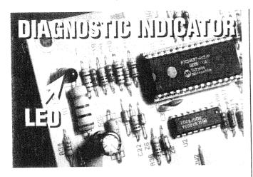
19. A light emitting diode (LED) on the IGC provides an indication when there is a fault in the unit or in the control itself. The LED remains on when the unit is operating normally and remains off when there is a major malfunction such as a loss of 24-volt power.
