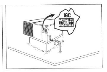
3. The IGC responds to inputs from any 24-volt central control or heating-cooling thermostat\*. This sophisticated control board makes the control of rooftop units more reliable. It also simplifies rooftop unit troubleshooting through its built-in diagnostic function.
