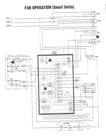
24. With the power on and the overcurrent protection closed, there is a path through J2-R to supply 24 volts to the thermostat and FAN switch. If the FAN switch, at 1, is set to ON, the indoor fan operates continuously. This switch provides a path through J2-G to the fan logic and blower relay BR, at 2, will be energized.
