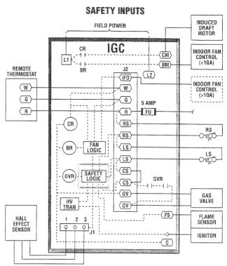
12. The safety logic receives inputs from the unit's rollout switch, limit switch, flame sensor, and the IGC fan logic. It also receives an input from the device used to prove operation of the induced draft motor, which can be either a pressure switch, centrifugal switch, or Hall Effect sensor. In this program we will use the Hall Effect sensor.
