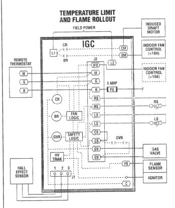
16. Terminals RS and LS on J2 connect the IGC safety logic to the unit's rollout and limit switches. If either switch opens, the safety logic shuts off the gas flow and energizes the unit's blower and induced draft fan to cool and purge the heat exchangers. In the event of a flame rollout the IGC also locks out the unit.
