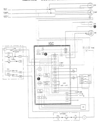
33. Forty-five seconds after the burners ignite, the safety logic signals the fan logic to energize the blower relay BR, at 1, closing the BR contacts, at 2, and energizing the indoor fan motor, at 3. As described in the Familiarization section, if the limit switch opens prior to the fan coming on, 5 seconds are subtracted from the fan delay. For example, if the limit switch trips after 38 seconds, on a relight the fan delay time is reduced to 33 seconds.
