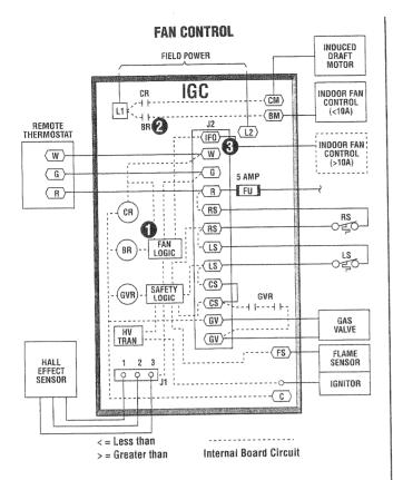
9. The fan logic, at 1, controls the timing of the indoor fan, also known as the blower, by controlling on-board blower relay BR contacts, at 2, or an external fan contactor for the larger size units. The blower relay can handle blower motors drawing up to 10 amps. If the unit being controlled uses a larger blower, the IGC will control the unit's indoor fan contactor through terminal IFO, at 3, on J2. More about this in the Operating Sequence Section.
