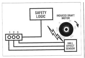
13. The Hall Effect sensor is a magnetic device mounted on the induced draft motor. As long as the motor is turning at the required speed, the sensor produces an induced current which signals the safety logic that the induced draft fan is running at the required speed.
