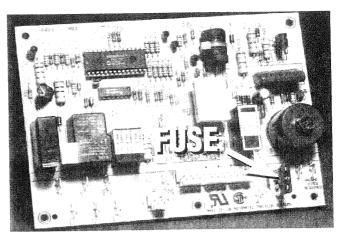
21. A 5-amp, automotive-type fuse on the IGC provides overcurrent protection for the remote thermostat and the secondary of the 24-volt transformer.
