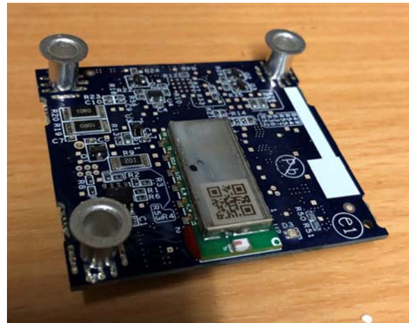
Fig. 25 – Bluetooth Module (used on all models)
