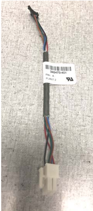
Fig. 30 – PCM to Bluetooth Module Comm Cable (used on all models)
