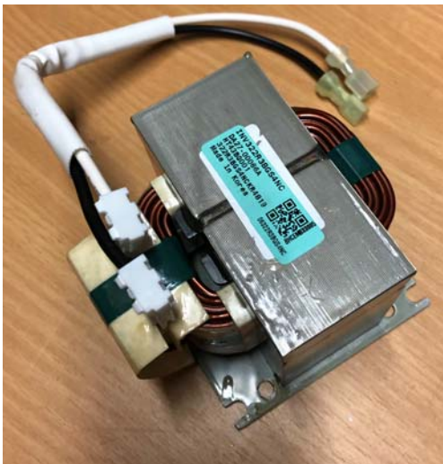
Fig. 27 – 2/3/4T Reactor (Note: 4Tuses 2 reactors)
