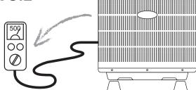
Refrigerant tubes and indoor coil should be evacuated using the recommended deep vacuum method of 500 microns.
