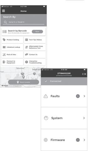
Available from Google Play® or the App Store®, our greatly enhanced Carrier Service Technician app will guide you through processes such as troubleshooting, Bluetooth pairing and even over-the-air software updates. It provides access to outdoor unit parameters such as system pressure, voltage for the system, compressor RPM and temperature.
