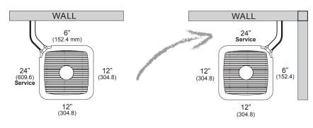
Allow 24 in. (609.6 mm) clearance to service end of unit, and 48 in. (1219.2 mm) above unit.
