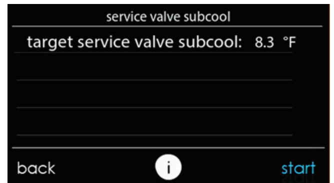
Fig. 14 – Liquid Service Valve Subcooling Target
